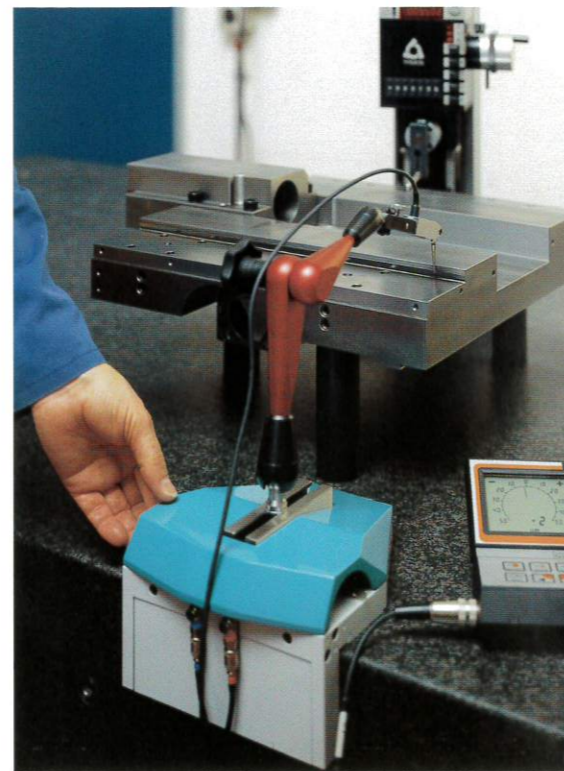
The measuring device „Straightline“ provides for angle and evenness measurement with maximum measuring accuracy.
